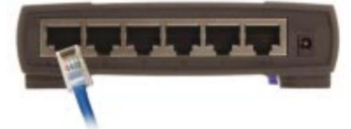
To connect a computer directly to the Switch, plug one end of the cable into any available port marked 1-5 on the back of the Switch, and then plug the other end of the cable into the computer's network adapter.
