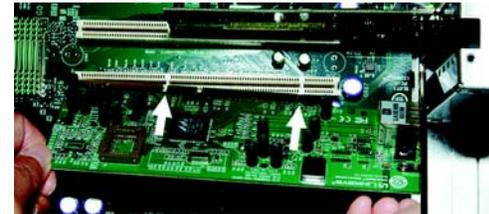
Figure 3-1: Insert the Adapter into the PCI Slot
