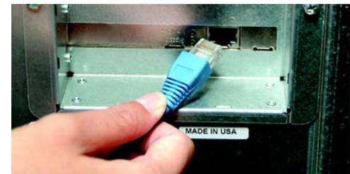
Figure 3-3: Connect the Ethernet Network Cable
