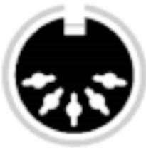
This is a 5-Pin AT keyboard connector. Use the PS/2-to-AT adapter.
