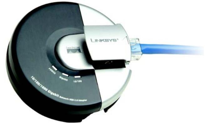
**Figure 2-3: Front Panel's Ethernet Port**
