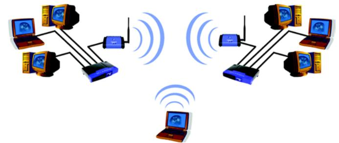
**Figure 2-3: Wireless Bridging Using Two Bridges**
