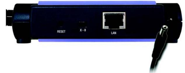
**Figure 4-2: Connect the Power Adapter**
