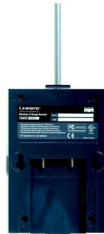
Figure 3-2: Recess for the Power Plate
