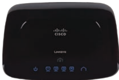
Power, Ethernet, and Powerline LEDs Light Up
