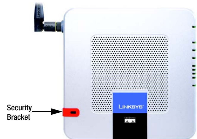
Figure 3-2: The Router's Front Panel
