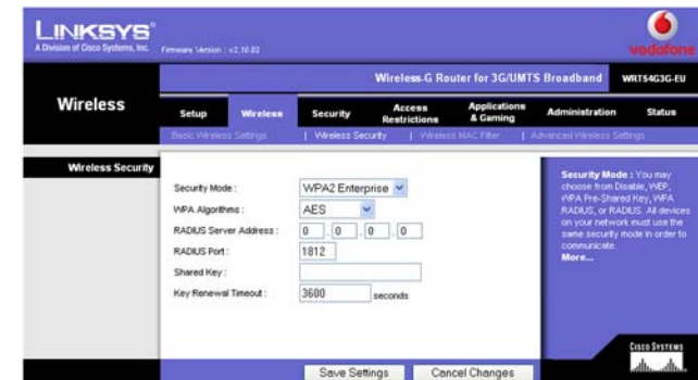
Figure 8-31: Wireless Tab - Wireless Security (WPA2 Enterprise - AES)
