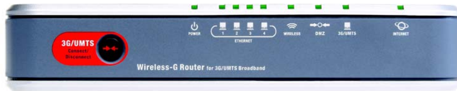
Figure 3-3: The Router's LEDs
