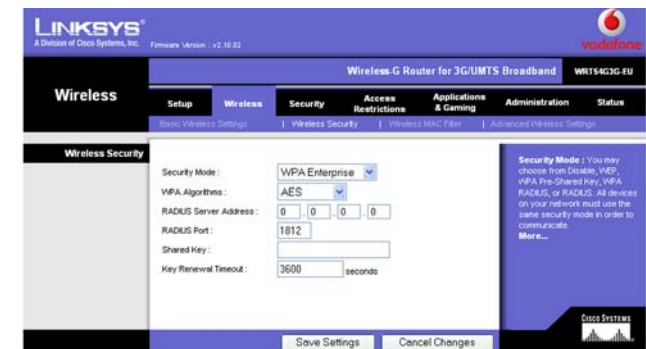
Figure 8-29: Wireless Tab - Wireless Security (WPA Enterprise - AES)
