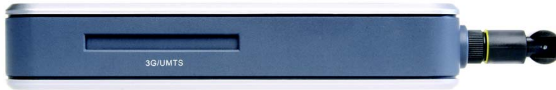
Figure 3-4: The Router's 3G/UMTS Data Card Slot
