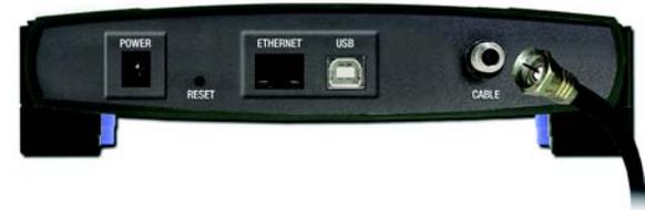
Figure 3-3: Connect the Coaxial Cable
