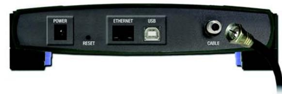
Figure 3-1: Connect the Coaxial Cable
