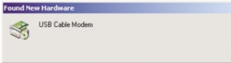
2. When the *Found New Hardware Wizard* screen appears to confirm that the USB Modem has been identified by your PC, make sure the Setup Utility CD is in the CD-ROM drive and click **Next**.
