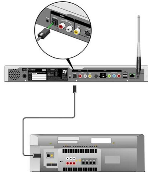
**Figure 3-6: Connect the Digital Audio Cable**
