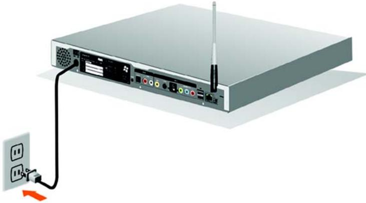
**Figure 3-7: Power on the Extender**
