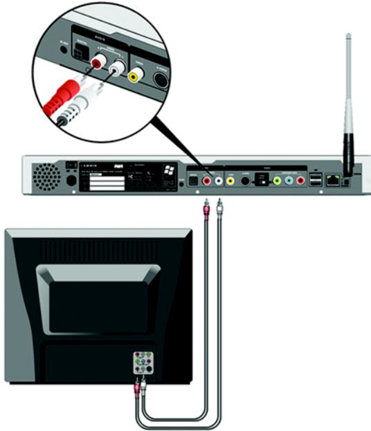
**Figure 3-5: Connect the Analog Audio Cables**
